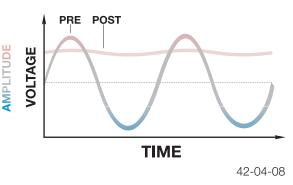
**Bosch LSH 25 Oxygen Sensors:** The post catalyst oxygen sensors produces a low voltage (0-1000 mV) proportional to the oxygen content exiting the catalytic converters.
